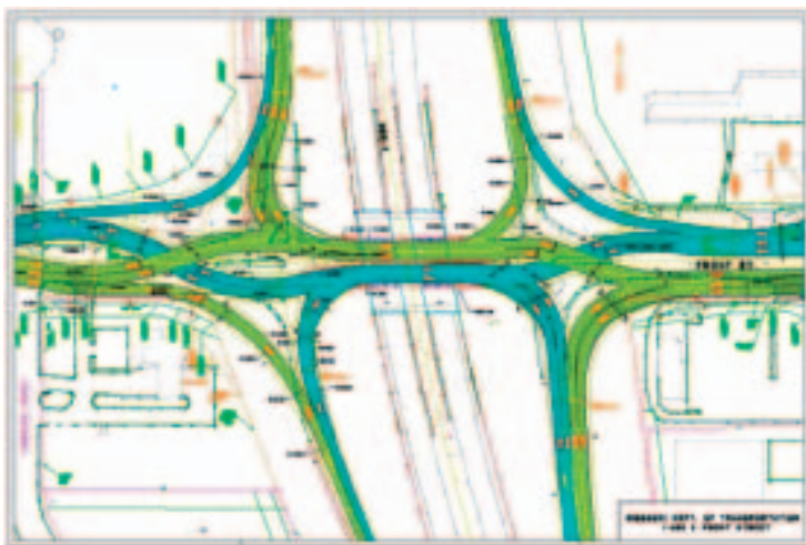
This figure, developed by the Missouri Department of Transportation, is the engineering drawing showing the proposed DDI at the I-435 and Front Street interchange on the east side of Kansas City. The traffic movements have been shaded in to more clearly show the opposing traffic movements.
