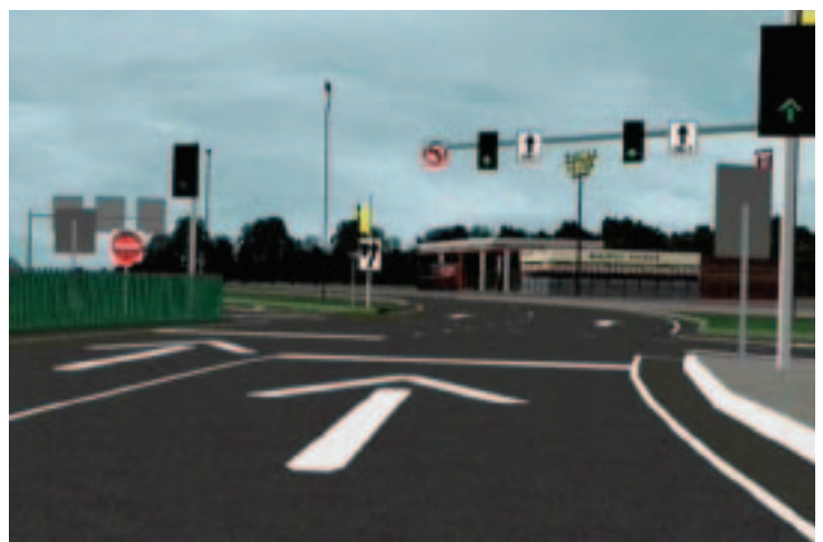
This screenshot of the FHWA simulation shows the driver's view approaching one of the traffic signals in the DDI. Note the placement of glare shields that block the view of oncoming headlights. Also note that the geometric design of the approach is meant to guide the driver to exactly where the driver should be, minimizing the possibility of a vehicle turning into oncoming lanes.
